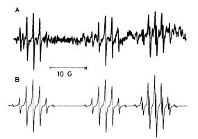
Figure. Low-field halves of 9.4 GHz e.s.r. spectrum of spiro[2.4]hex-2-yl radicals at 140 K. Upper trace (A) experimental; lower trace (B) computer simulation. Some lines from the rearranged radical, cyclobutenylethyl, can also be observed
